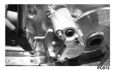
■ NOTE: Changing one pad at a time will prevent one piston from pushing out the other piston from the caliper.
