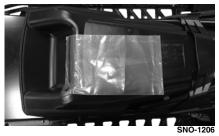
3. Slide the rear of the seat cover with foam over the rear of the gas tank; then slide the four tabs into the four holes in the lower console and secure to the tunnel using two selftapping screws. Do not over tighten. ■ NOTE: To ease the installation of the seat cover, carefully pry up the rear of the gas tank so the seat cover can easily slide around the rear of the gas tank.
