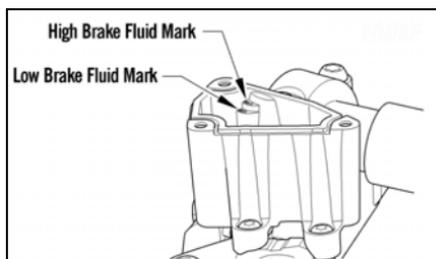
2. If the brake fluid is below the high brake fluid mark, add Arctic Cat approved DOT 4 brake fluid until the fluid is at the recommended level. Install and secure the reservoir cover. Do not allow moisture to contaminate the brake system.
