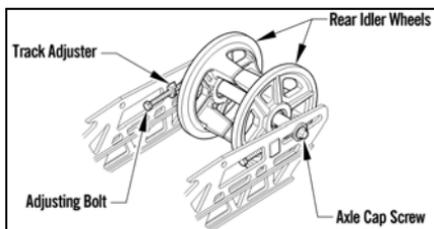
2. Check track alignment and continue adjustment until proper alignment is obtained.
