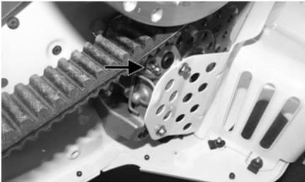
3. Slowly compress the brake lever until maximum pressure is attained; then hold the lever in the compressed position to maintain pressure. Open the bleeder valve to release the fluid and air. When the fluid stops, close the bleeder valve; then release the brake lever.
