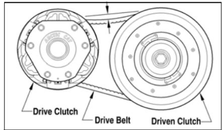
The drive belt must have the proper fit in the drive clutch and driven clutch. To check for proper drive belt fit, use the following procedure.
