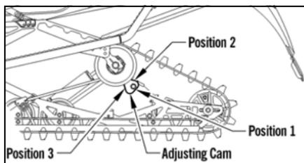
To rotate an adjusting cam, use the spark plug wrench from the tool kit. Rotate the wrench until the cam is in the desired position. To stiffen the ride, rotate the cam so as to raise the spring end. Make the appropriate adjustment on the other cam.
