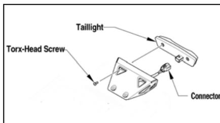
2. Remove the two torx-head screws securing the taillight to the bracket.
