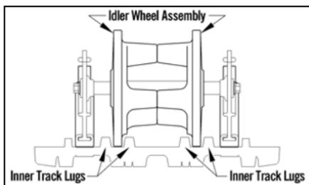
5. If the idler wheels are not centered between the inner track drive lugs, an adjustment is necessary.
