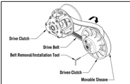
3. When the sheaves are fully apart, pull up on drive belt and roll belt over stationary sheave until it is free of the driven clutch.
