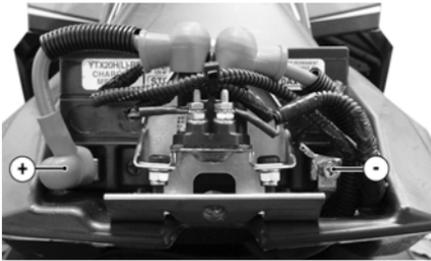
12. Install the battery bracket/solenoid and tighten the two screws and lock nuts to 105 in.-lb; then install the seat and secure with the torx-head screw. Tighten securely.
