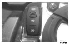
This switch allows the operator to operate the vehicle in either two-wheel drive (rear wheels) or four-wheel drive (all wheels) as well as mechanically lock the differential (if equipped) to apply equal power to both front wheels. For normal riding on flat, dry, hard surfaces, two-wheel drive should be sufficient. In situations when additional traction is necessary, four-wheel drive would be the desired choice.
