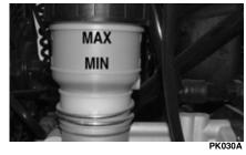
1. Check the brake fluid level in the brake fluid reservoir. The fluid level must be maintained between the MAX and MIN level marks. If the level in the reservoir is low, add
