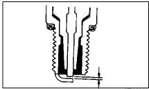
A new spark plug should be tightened 1/2 turn once the washer contacts the cylinder head. A used spark plug should be tightened 1/8-1/4 turn once the washer contacts the cylinder head.
