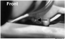
4. After all the oil has been drained, install the drain plugs and tighten to 45 in.-lb (5 N-m).
