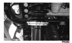
■ NOTE: Before attempting to adjust suspension, clean dirt and debris from the threads and remove load from the suspension; then use the spanner wrench to adjust the preload.
