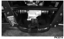
This vehicle is equipped with a rear frame-mounted receiver for a standard 5.1 cm (2 in.) receiver hitch. The standard receiver hitch must be purchased separately.
