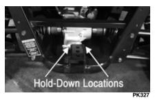
■ NOTE: Suitable hold-down straps are available from your authorized dealer. Ordinary rope is not recommended because it can stretch under load.
