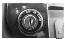
**OFF** position — All electrical circuits except the accessory are off. The engine will not start. The key can be removed in this position.
