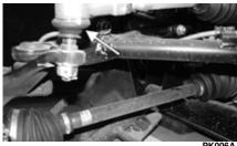
5. If boot damage is present or tie rod end free-play seems excessive, contact an authorized dealer for service.
