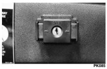
3. To open the tailgate compartment, pull outward on the locking lever and allow the tailgate storage cover to pivot downward. To secure the tailgate storage cover, pivot the cover upward and press firmly on both left and right hands sides.
