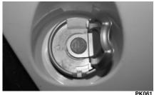
2. After filling the tank, position the lid toward the right side of the filler neck and rotate the lid 1/4 turn clockwise to secure. Flip the lid up.
