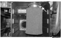
3. Remove the Phillips screw to separate the air filter holders from the air filter.
