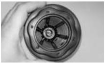
MOD089 7. Remove and inspect the safety filter.
