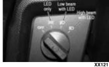
Use the headlight switch to select the LED light strip, low beam with LED or high beam with LED. When the switch is in the LED position only, the light strip will illuminate. When the switch is in the low beam position, the low beam will illuminate along with the LED light strip. When the switch is in the high beam position, the high beam will illuminate along with the LED light strip.
